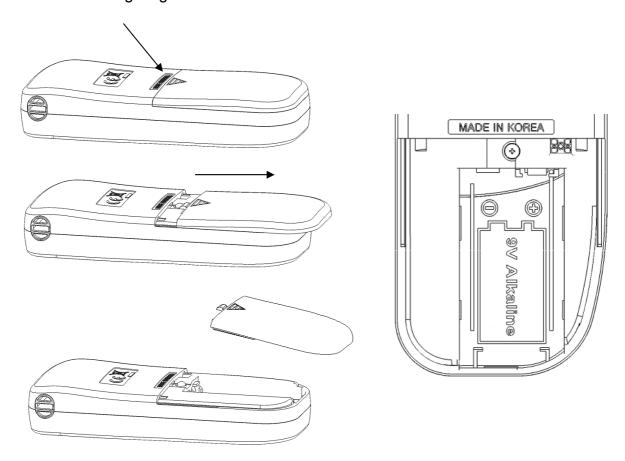
\*\*\* N.B. : Make sure to insert the battery with the proper position of positive(+) and negative(-) as indicated.
