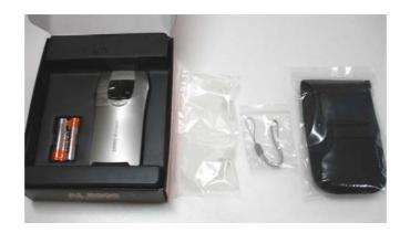
The AlcoScan AL-5000 analyzes a breath sample to detect alcohol in the lungs. This reading is then converted to blood alcohol concentration (BAC). The AlcoScan AL-5000 uses an advanced oxide semiconductor sensor to detect alcohol. It also features replaceable mouthpieces.
