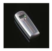
The AlcoScan AL2500 analyzes a breath sample to detect alcohol in the lungs. This reading is then converted to blood alcohol concentration (BAC). The AlcoScan AL2500 is very convenient and portable. No mouthpiece is required.
